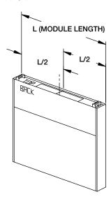
If the back supply plenum is greater than 9 ft. 10 in. (299.72 cm) long, divide the length of the back supply by four. This will give you the center of each half. Cut openings at the suggested location, centering the duct collar over the center measurement of each half.
